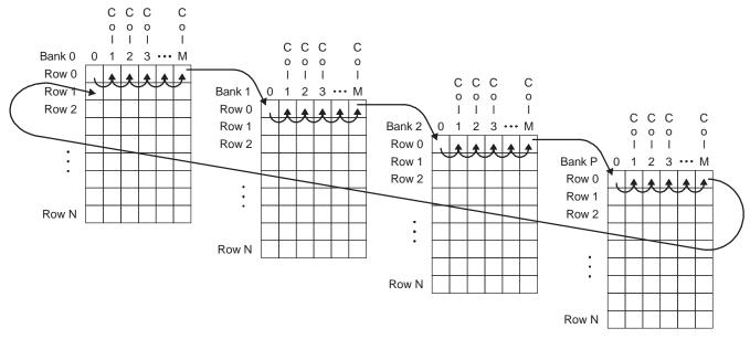
Figure 14. DDR2 SDRAM Column, Row, and Bank Access
